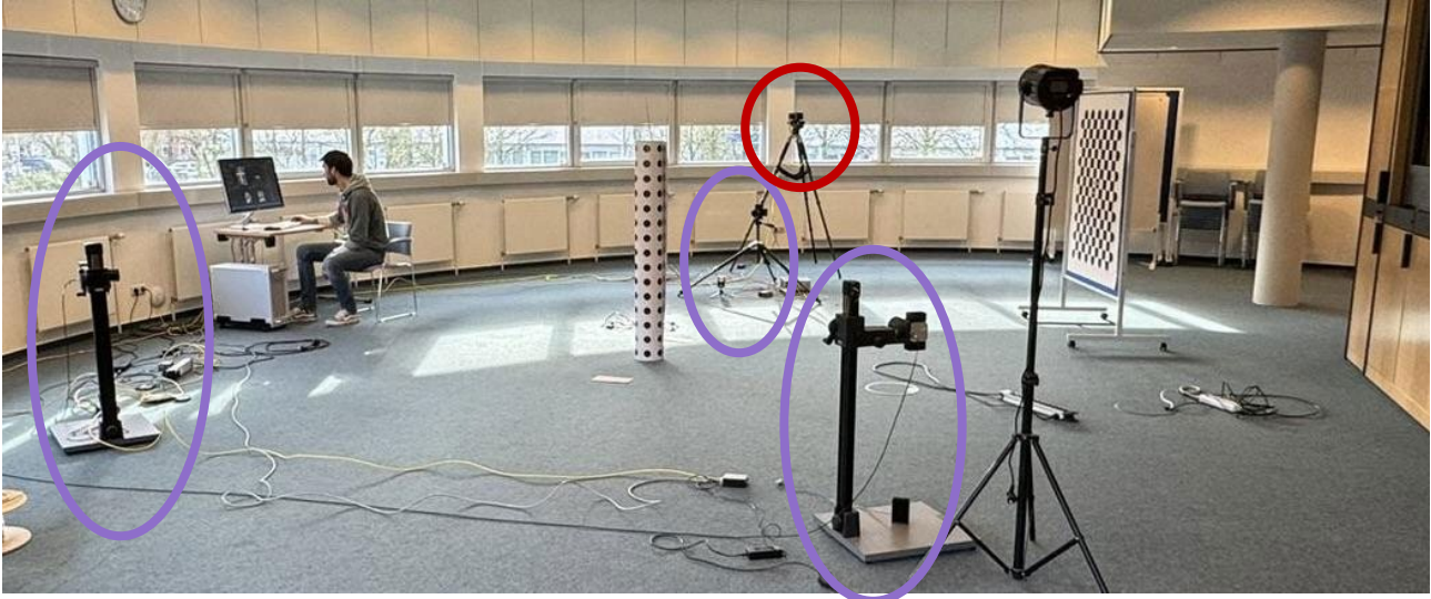
Figure 4: Multi-camera setup built with Raytrix R32 cameras and an edge computing system
