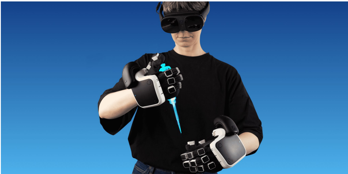
Figure 4: SenseGlove Nova 2, force and haptic feedback glove used within PRESENCE.
