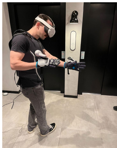
Figure 1: PRESENCE's developer testing the first implementation with both the SenseGlove Nova 2 haptic gloves and the Skinetic haptic vest.
