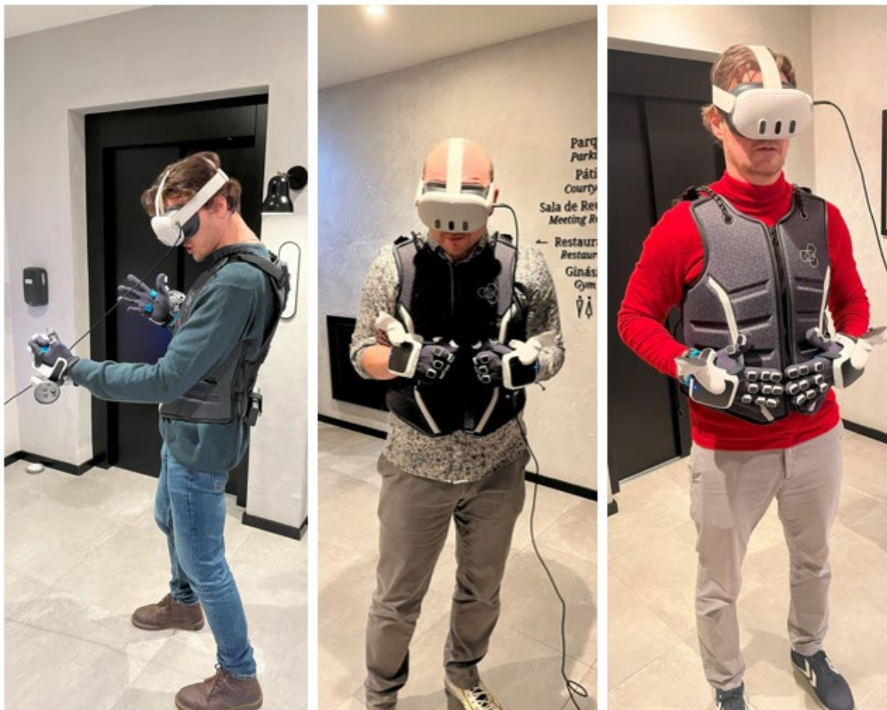
Figure 19: Users immersed in a VR scene using SenseGlove nova Haptic gloves and Actronika's Skinetic vest
